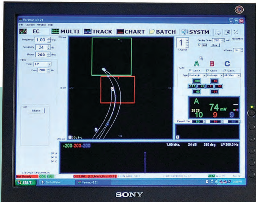
The Varimac® monitor screen displays rectangular targets that show “acceptable” parts in the green box, “above spec” in the red box, and “below spec” outside the boxes.
