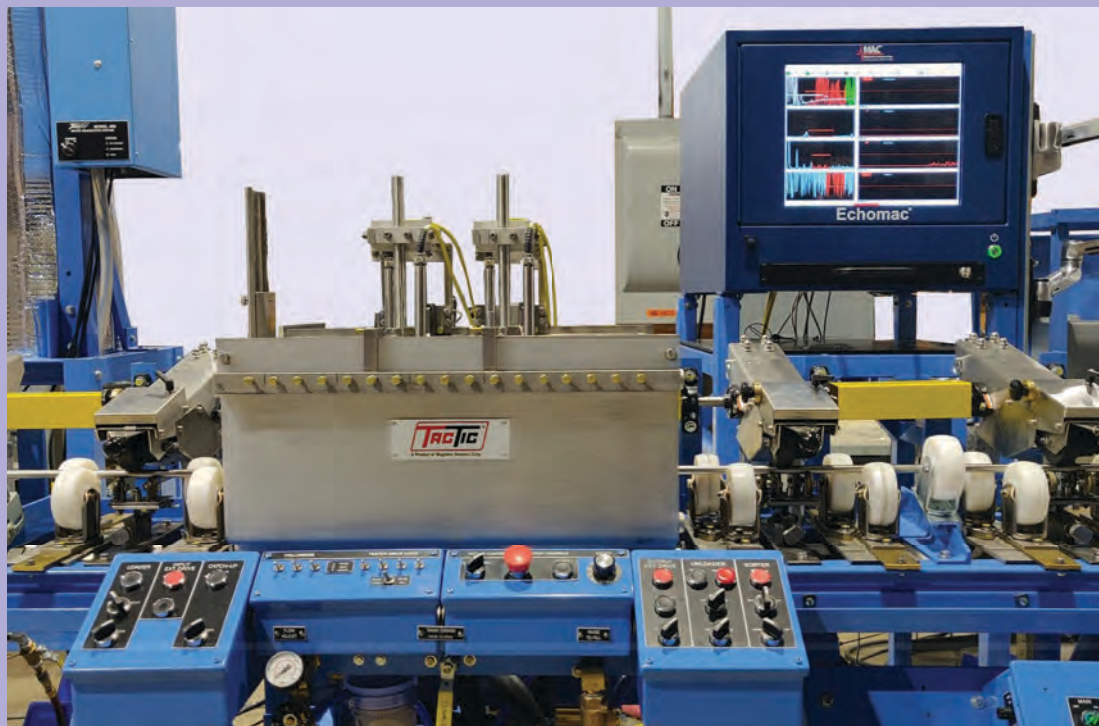
MAC’s Echomac® FD 6A ultrasonic instrument with TacTic’s® standard heavy duty “Spin The Tube” Immersion-Style System to test titanium tube.
