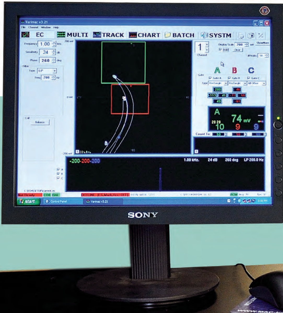
The Varimac® monitor screen displays rectangular targets that show “acceptable” parts in the green box, “above spec” in the red box, and “below spec” outside the boxes.
