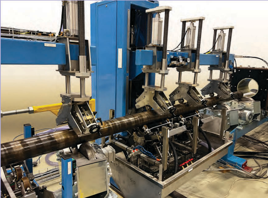
A Spinning Tube Full Body Ultrasonic test system for detecting longitudinal and transverse flaws, wall thickness, and lamination in ERW cold drawn carbon steel tube.
