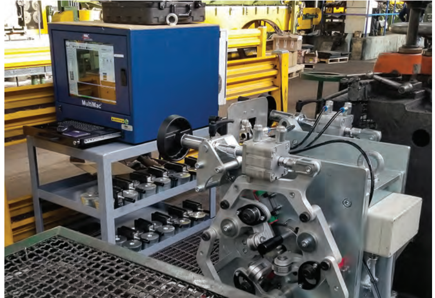
MultiMac® Eddy Current Tester inspects hex and round bars on a Schumag line. A CP 65mm “floating” Coil Platform with pneumatically loaded triple guide rolls is in the foreground.
