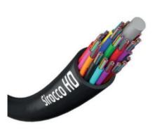
The SE 864f microduct cables employ state-of-the-art BendBrightXS 180 µm single-mode (ITU-T G.657.D, G.657.A2) bend-insensitive fiber that ensures compatibility with existing G.652 fibers and readiness for evolved systems. They are available in fiber counts ranging from 96 to 864 and conform to interna-
