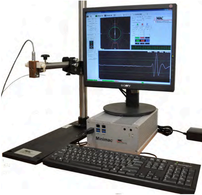
XWNE3 XSB (extra small body) High Frequency (3MHZ) test coil screen showing a defect in a Nitinol standard wire.
