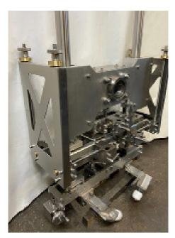
An electric motor raises and lowers the follower to accommodate changes in test material diameter. An air cylinder is used to raise and lower the follower for a small distance above the test material to permit rapid bridge motion along the tank length as desired. An adjustable "stop bar" prevents the follower from dropping if it runs off the end of a test piece.
