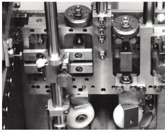
The TACTIC™ model 411 dual probe follower has been in service for many years. This follower allows the transducers to ride a test piece to assure a constant angular relationship to the tube or bar as it rotates. Downward (following) pressure can be provided by gravity, or by regulated pneumatic pressure. See TACTIC™ bulletin 4110 for more basic details.
