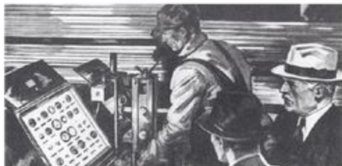
In the June 3, 1940 issue of Time Magazine, this ad from Jones & Laughlin Steel Co. shows an electromagnetic MAC tester for inspecting cold-drawn bars. © Magnetic Analysis
