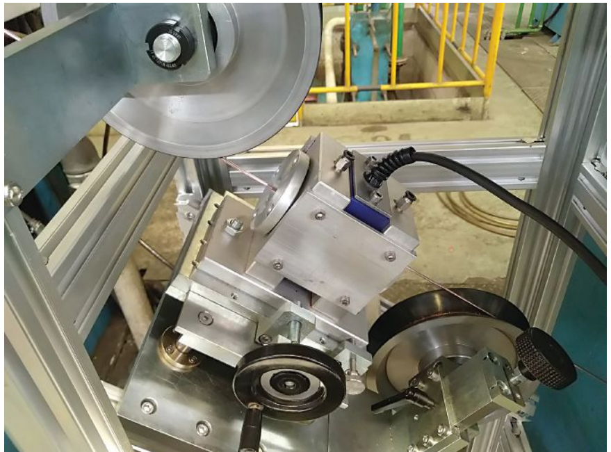
MultiMac® eddy current blue test coil in holding and guiding mechanism from Ningbo NewDev Optoelectronic Technology Co., for testing rod or wire during production.
