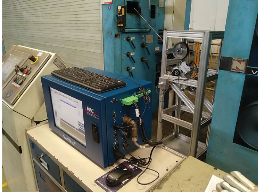
MultiMac® eddy current tester and Ningbo NewDev Optoelectronic Technology Co.'s enclosure and guidance mechanism for testing rod or wire during production.
