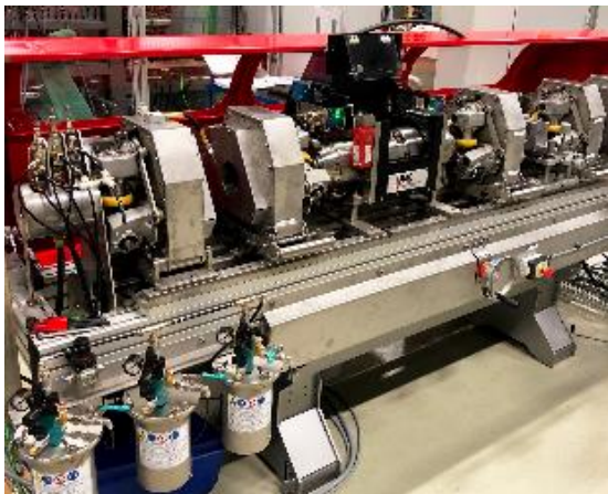
Echomac® 25mm ultrasonic rotary on a test bench for inspecting small diameter material.
