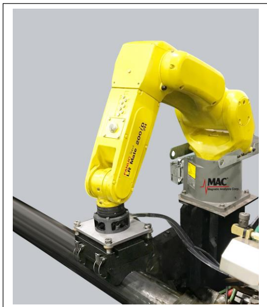
Magnetic Analysis Corp.'s Turnkey Phased Array Ultrasonic System for Inspecting ERW Tube
