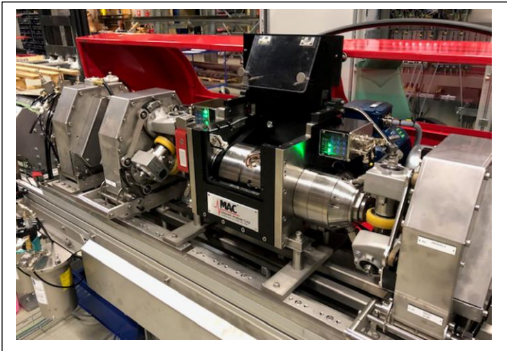
Echomac® 25mm Ultrasonic rotary for inspecting tube and bar
