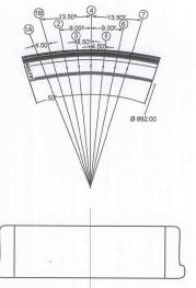
NOTE: ALL MEASUREMENTS ARE IN MILLIMETERS. HOLES 2-5 ARE COUNTERBORED AT 3.3mm Ø \*SDH 1B IS VOID DUE TO DRILL REMAINING INSIDE OF HOLE.
