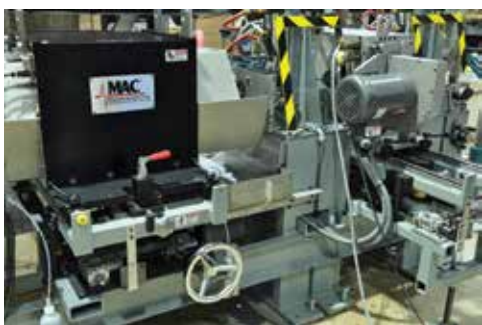
Part of a 50mm Ultrasonic and Eddy Current system to test bar for automotive applications, meeting Mil Std Class B, Class A and some Class AA levels, finding surface defects one percent deep.
