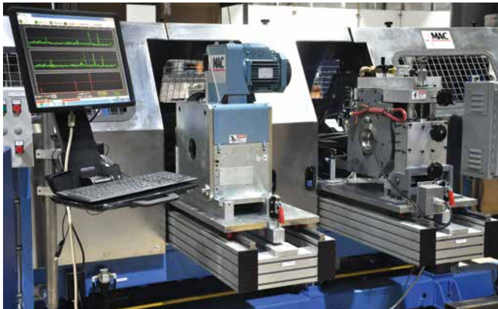
Part of a stand-alone eddy current test system for bar 3/4" to 3 1/2" diameter in Illinois. The system includes a rotary probe tester, shown at center, and encircling coil eddy current unit, at right.
