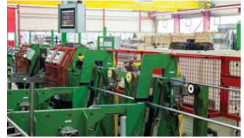
A Magnetic Analysis Corp. Echomac® UT system and conveyors at Schoeller Werk GmbH inspects stainless steel heat exchanger tube. Part of the important mechanical support for the tube as it enters the test is shown in the foreground.
