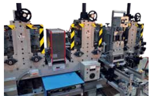
An Eddy Current system to test 2" to 6" diameter ERW tube for weld zone defects such as penetrators includes a Multimac® instrument, water cooled encircling test coil, demagnetizer and Dual Pinch Stands.
