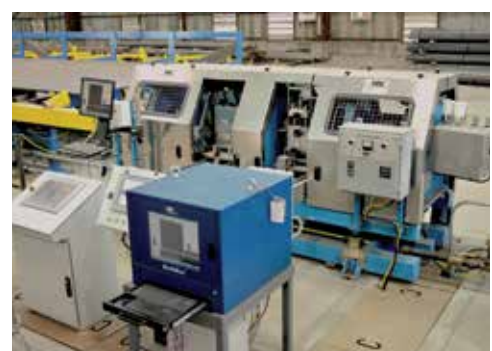
Eddy Current stand-alone system on a triple drive roll bench for testing bar. The system includes an encircling test coil, a rotary probe test unit, and the Multimac® electronics.
