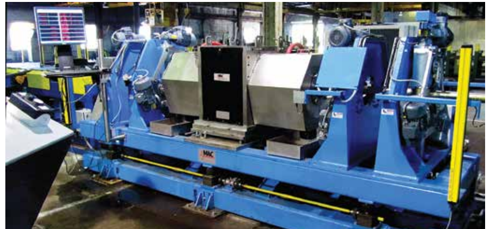
A stand-alone ultrasonic system to inspect bar, mounted on a triple drive roll bench.
