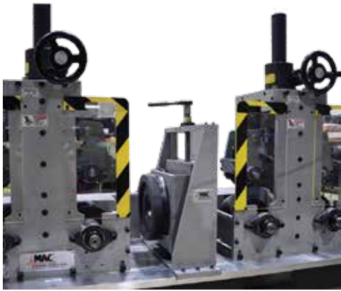
An Eddy Current Coil Platform and drive with a special bushing to handle TIG welded Austenitic stainless steel 300 series tube as it passes through the test coil.
