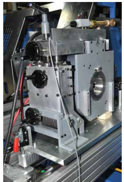
An eddy current encircling coil for use in a system to test steel bar 3/4"-3.5" diameter.
