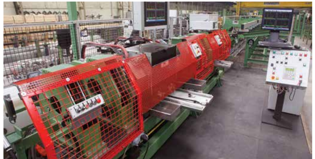
This MAC Echomac® Ultrasonic system inspects stainless steel heat exchanger tube at Schoeller Werk GmbH. MAC also designed and supplied the conveyor system which helps ensure accurate testing.
