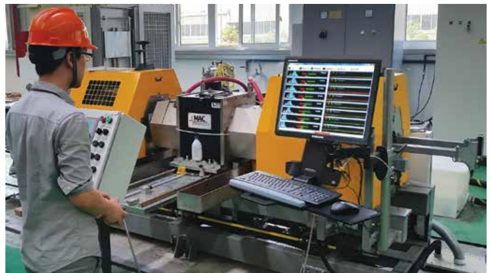
Miles Jing, MAC's Chinese Field Engineer, checks out a new 50mm Echomac® Ultrasonic rotary at a customer's plant to test ERW pipes destined for automotive parts.
