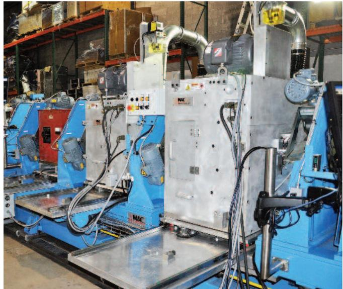
*Longitudinal & transverse flux leakage rotaries, ultrasonic rotary, and demagnetizer multi test system.*
