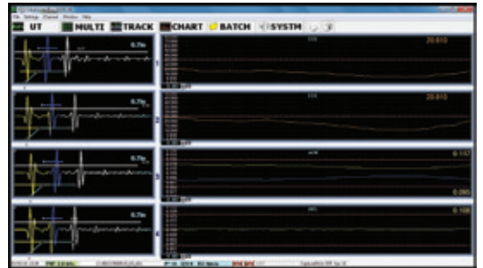
Instrument display showing A-scan of each thickness measurement, as well as charted data of two separate eccentricity alarms, min and max wall, and average wall
