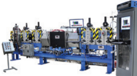
The multi-test system for automotive shock absorber tubing and OCTG features 100mm ultrasonic Echomac rotary test and a MultiMac eddy current tester
