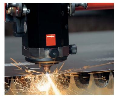
recision laser cutting specialist FC Laser has installed a new 10kW Bystronic fibre optic laser centre which is capable of cutting materials as thick as 30mm with incredible accuracy. Two more identical machines are to be ordered over the coming months.
