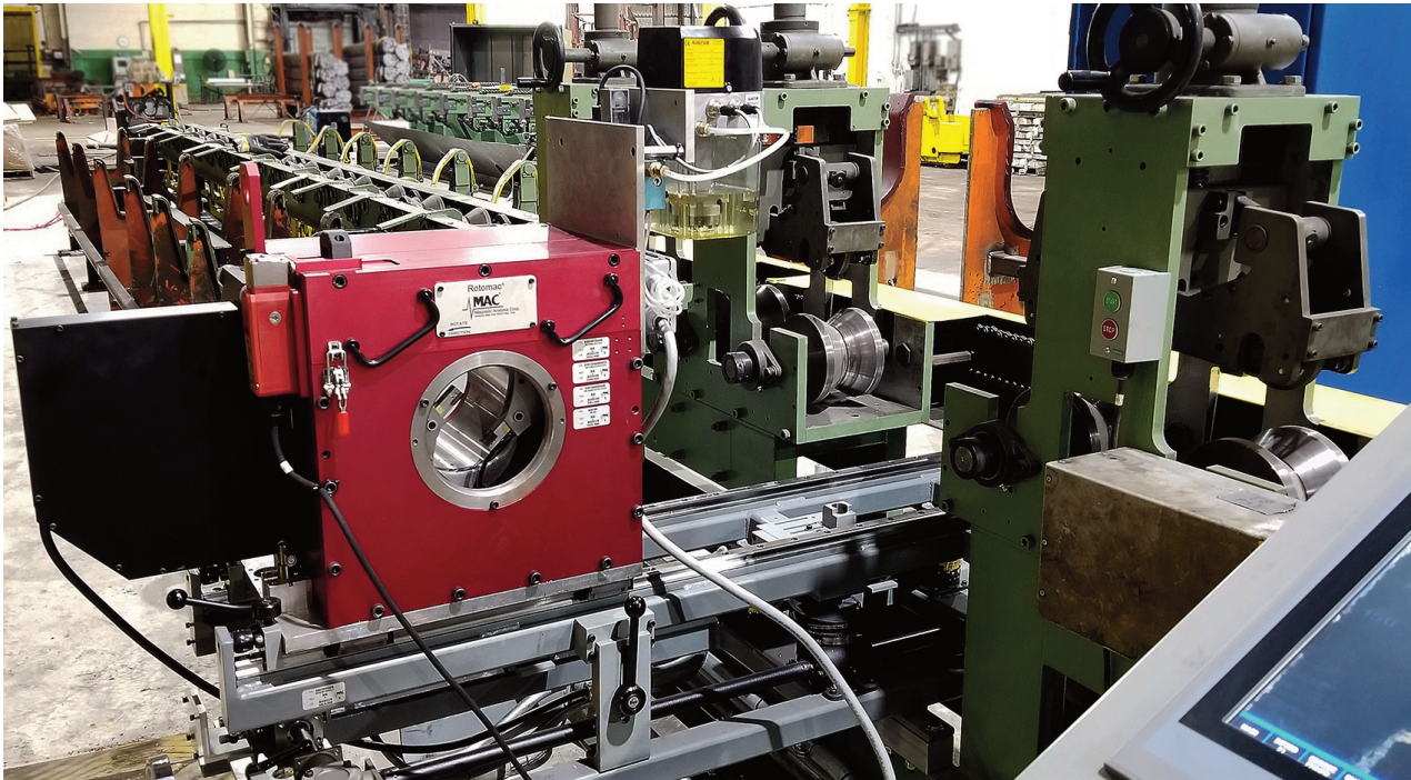
An Eddy Current Rotomac® 150mm rotary inspects cold finished bars at a US mill.
