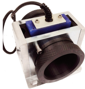
65 CP nonsaturating coil platform with a 4" x 5" test coil inserted
