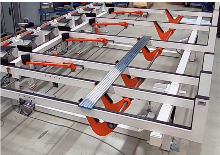
Adjustable Stop Arms are in the "full-up position when a bundle of material is placed on the feed rack, they are then lowered gradually, controlled by an electrically operated air valve, to allow a limited number of bars to spread out on the feed racks.
