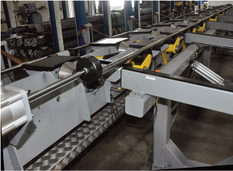
The aligner disk is seen above pushing the bar to the correct position to be fed to the accumulation table.
