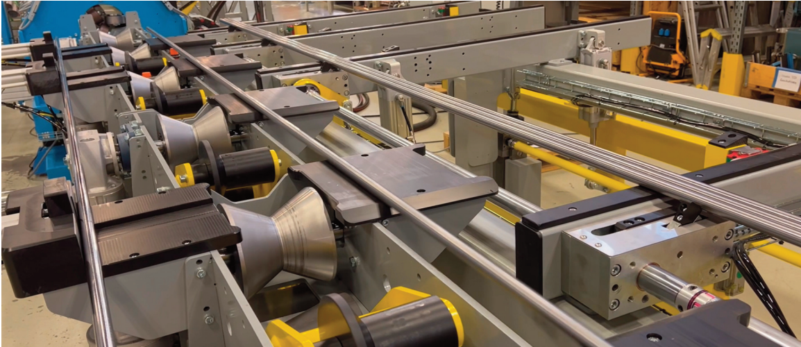
Pneumatic release mechanisms retain the material on the rack and release the bars individually to the Easy Drop release units which raise and lower the bars onto the Channel Roll Sections that feed the material into the tester.
