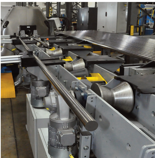
A sample bar rests on the custom calibration station which transfers the bar to the Channel Rolls to be run through the tester, then automatically reverses the bar and returns it to the station.
