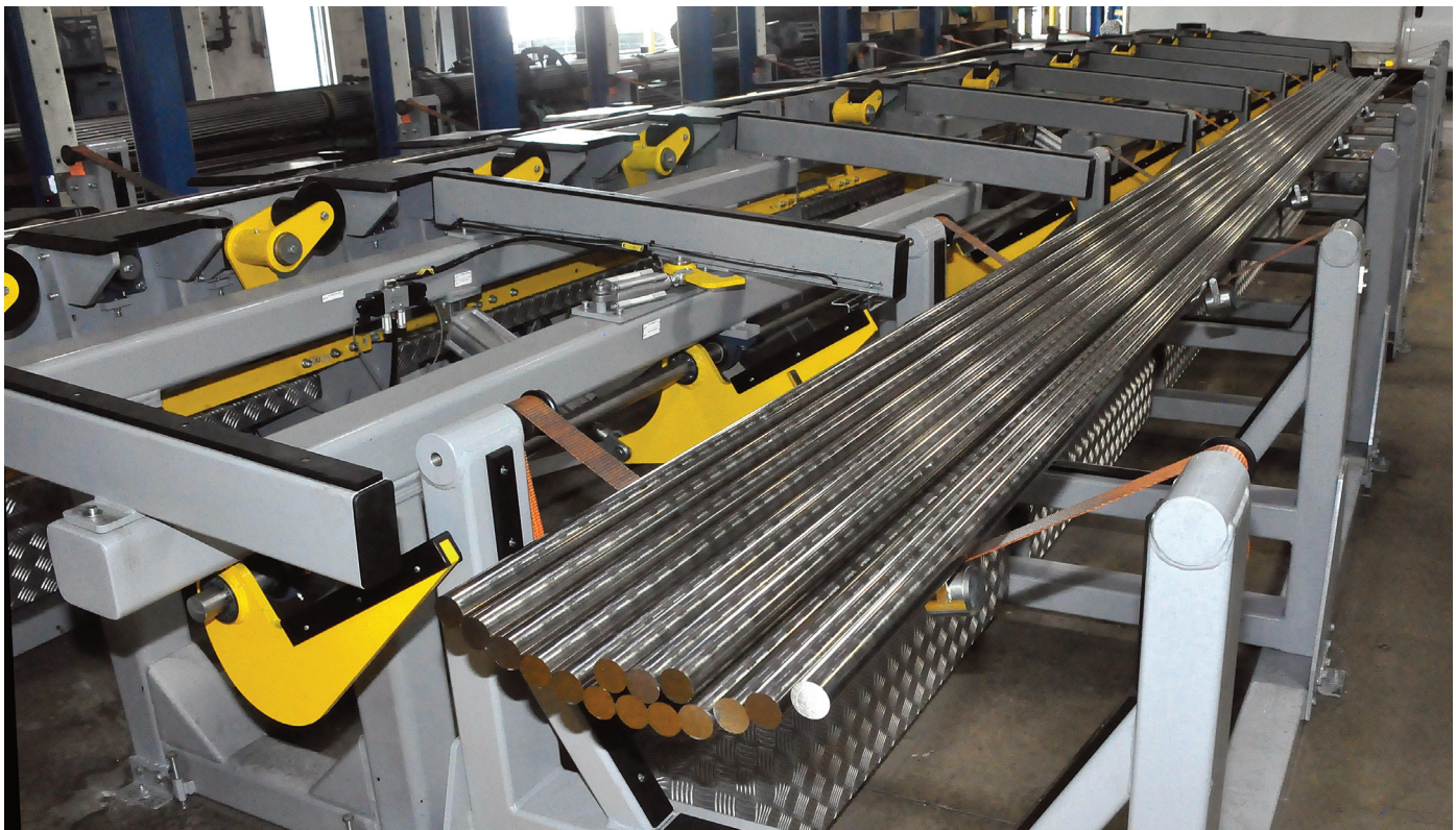
Accepted bars or tubes are released from the output table by stop arms into the receiving pockets which lower gradually as the quantity increases.
