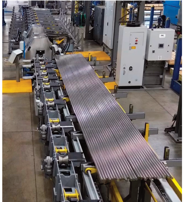
A bundle of bars spread out on a feed table, awaiting transfer to the channel roll conveyor sections, shown at left.
