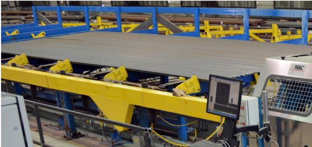
This rotary and coil eddy current system was designed to inspect SBQ steel from 0.750" - 3.5" diameter directly after the straightening process. The material is lifted onto the feed system which includes Release Mechanisms, Intermediate Stop Arm Attachments, and E-Z Drop Channel Section Loading Attachments-all within a programmable controller.
