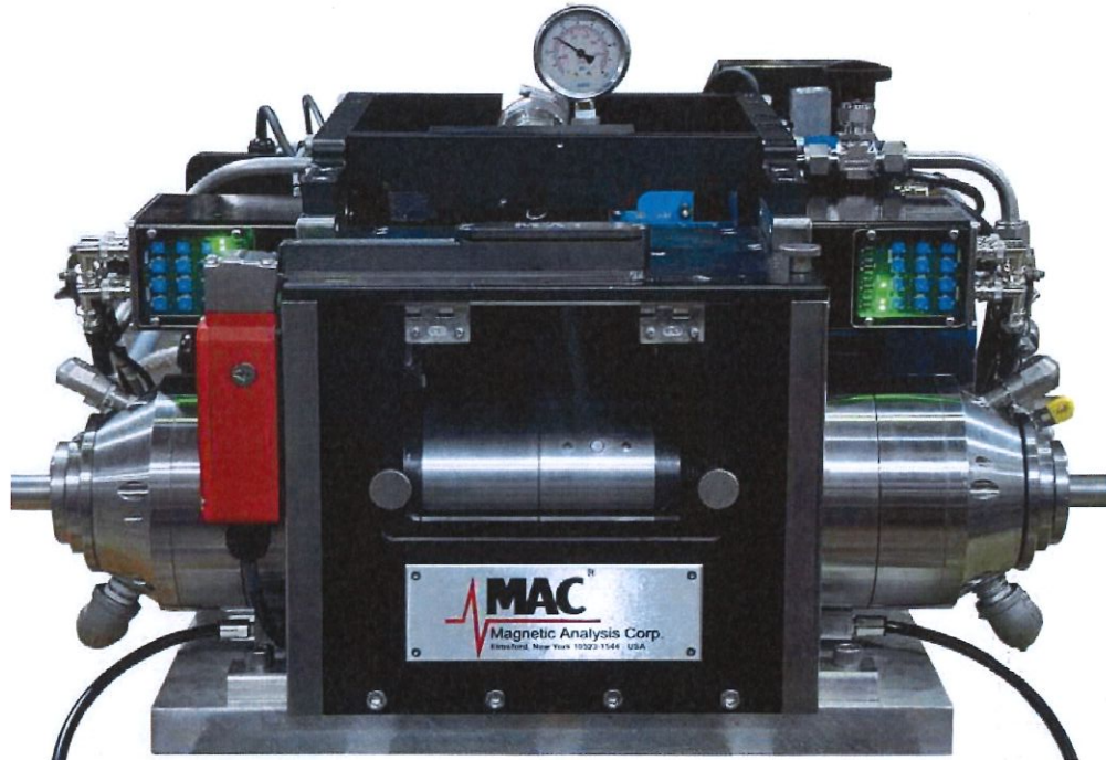
Echomac® 25mm Ultrasonic Rotary Tester for small diameter tube
