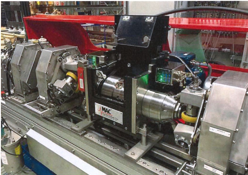
Echomac® Ultrasonic system, featuring 25mm UT Rotary for testing small diameter bar
