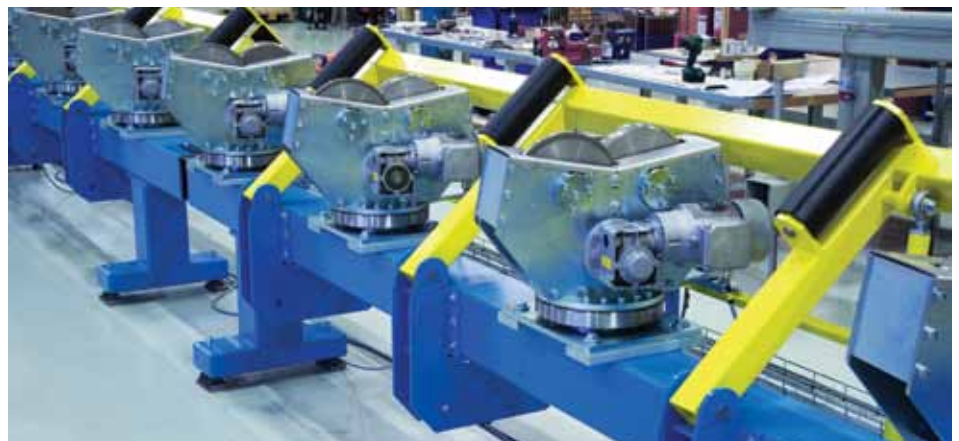
A custom designed helical spinning conveyor system ensures accuracy as tubes are fed into MAC's new APC (Automatic Pitch Control) full body ultrasonic tube tester.
