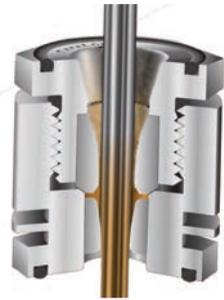
These dies vary greatly in their diameter, guide entry angle, materials, and hardness. The Varimac® sorts out dies with cracks that could cause extensive damage to equipment and substantial down time.
