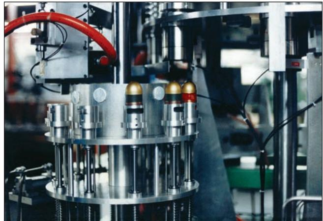
To inspect live grenades, this test system used robotic methods, operating behind a concrete wall to position the grenades for accurate and safe testing of longitudinal and transverse defects.
