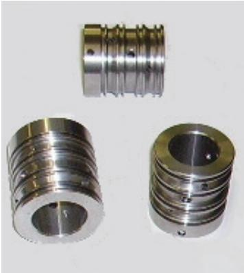
MAC uses its highly focused spinning probe eddy current technology to spot precision ground automotive parts such as fasteners inside the rotary. The probes test the "lands" in the parts (shown below) for seam detection.
