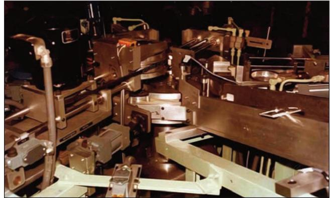
A large flux leakage and eddy current tester was designed and installed by MAC to inspect military ordnance such as shell bodies, shown above, using three separate stations; a load station, a test station, and an accept/reject station. Two flux leakage tests were used for transverse and longitudinal defects, and eddy current tests for cracks and hardness included the Varimac® and the Production Comparator.
