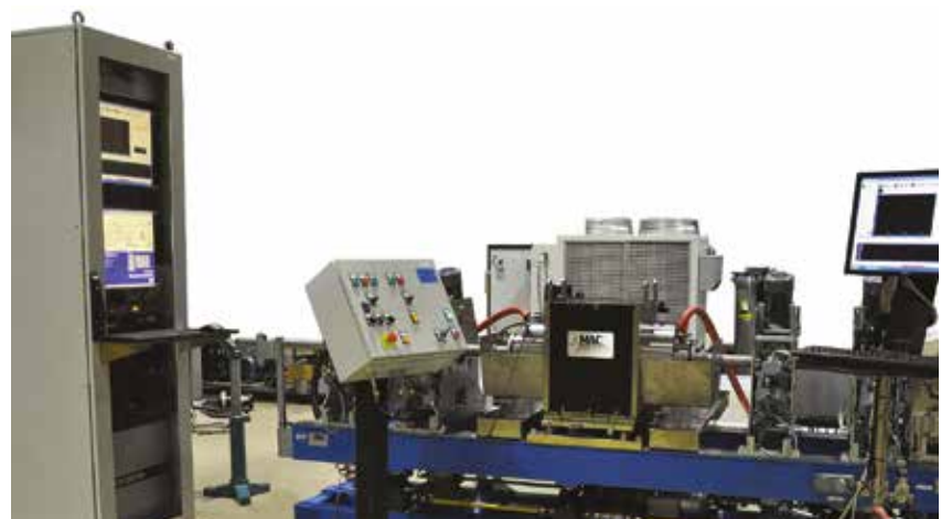
Echomac® Ultrasonic test system for inspecting welded stainless steel tube at Ratnamani Metals & Tubes Ltd., a major stainless tube producer in India for critical heat exchanger tube. The system detects transverse and longitudinal defects and measures wall thickness, ID and OD dimensions.
