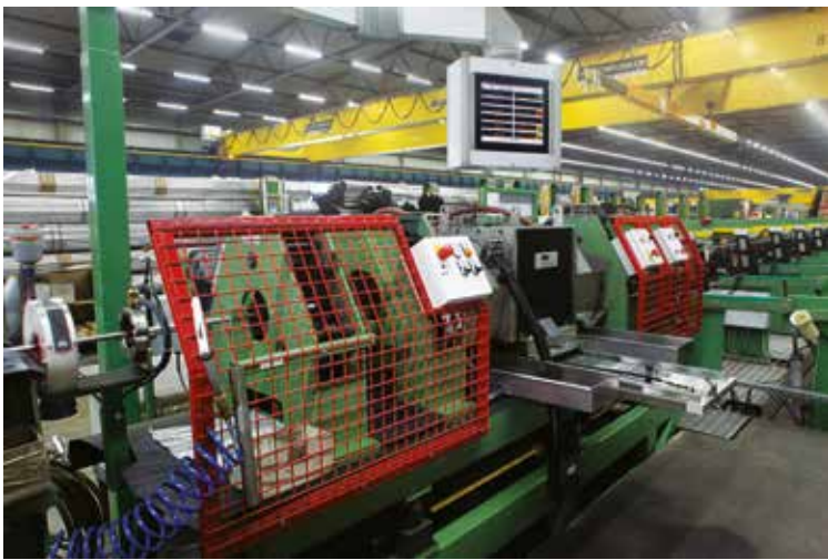
Echomac® Ultrasonic test system inspecting stainless steel and titanium alloy heat exchanger tubing for at Schoeller Werk. The test rotary is the black unit beneath the monitor.
