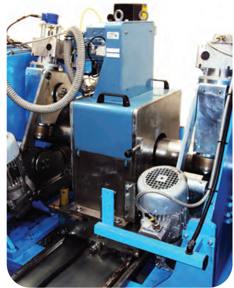
Rotary Probe Tester , shown above, used with MultiMac electronics to inspect hot rolled bar from 50mm to 150mm diameter. This multi test system is mounted in a triple guide roll bench and also includes an Echomac® ultrasonic tester.
