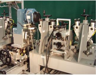
An installed eddy current system using a Rotomac® Rotary, at left, and an encircling test coil, in the center. Pinch stands at either end ensure the bar is positioned firmly and accurately for the test.
