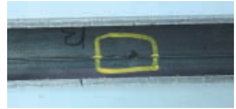
Figure 6 Eddy current methods can detect very short flaws, such as this pinhole, which are not normally detected by ultrasonic equipment.
