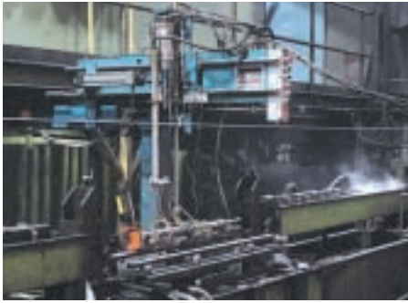
Figure 4 This ultrasonic test apparatus tracks the weld of the tube.
