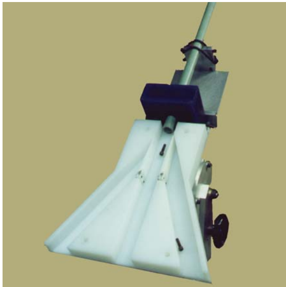
Model 570 Parts Gate, used with a vibratory bowl or other mechanics, feeds the parts through the test coil and into the correct one of three chutes for separating into above spec, below spec, and within specifications.
