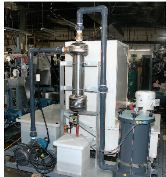
Recirculating water chiller systems that can be integrated with the Echomac UT rotary operation to provide clean, temperature controlled couplant for UT testing.
