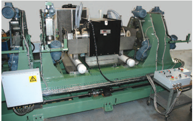
Echomac® UT-500 Rotary Ultrasonic System to inspect steel bar, mounted on a 125 mm Triple Drive Roll Constant Center Bench
