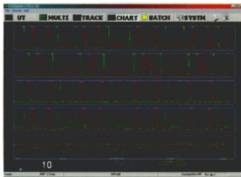
Figure 3 – screen display for a 20-channel Echomac® UT system to test 30ft-long, 3-6" diameter drill pipe for flaws and wall thickness. All data from 20 channels are consolidated into 5 channels for convenient viewing (courtesy Smith Services)
