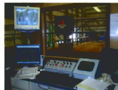
Figure 4 – control room with 20-channel UT screen display of drill pipe test data. Test electronics and transducers can be observed through the window (courtesy Smith Services)
