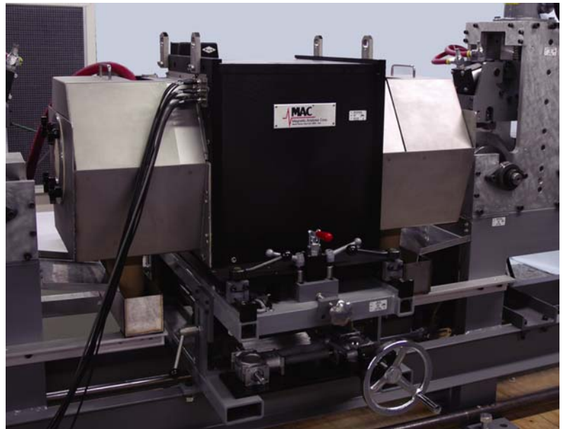
MAC Echomac 7 channel ultrasonic rotary mounted on an elevating platform, for inspecting 4" (101.6mm) diameter material. Rotating transducers are housed in the black enclosure, which also contains the pressurized water couplant.
