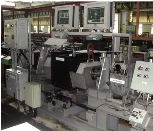
Tube inspection using an Echomac Ultrasonic Rotary mounted on an elevating platform, Demagnetizer to remove residual magnetism, and a MAC series Eddy Current encircling coil test.
