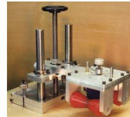
CP90 features a tangent coil and guide rolls on either side to maintain proper position of the material
