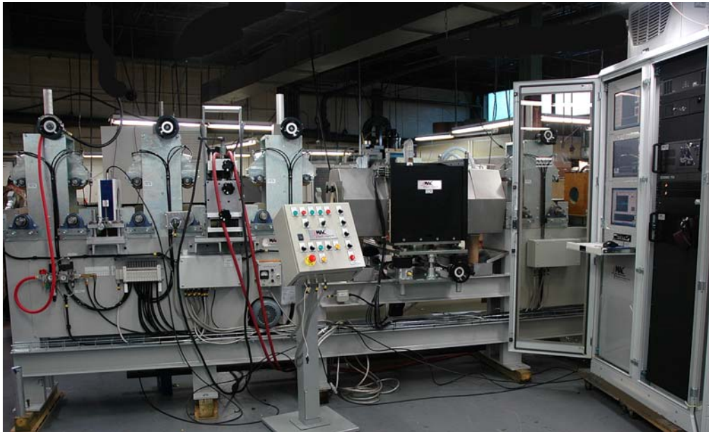
The picture above depicts a multitest system for inspecting welded tube using an Eddy Current Rotary & Encircling Coils Test, an Ultrasonic Rotary Test, & Demagnetization.
