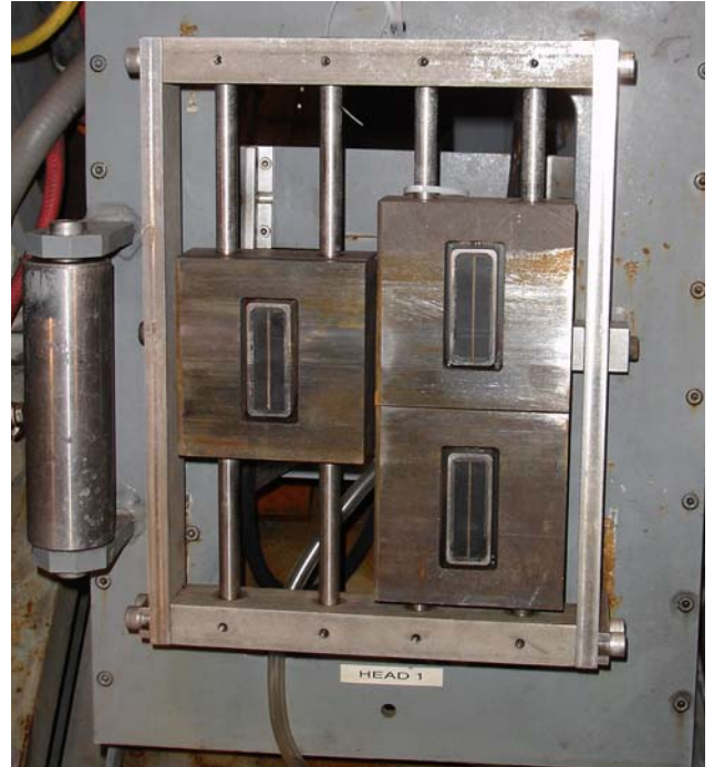
Test Head in Billet Testing Configuration
