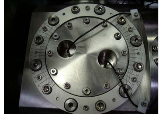
Shear wave mode transducer holder, with simple offset mechanism shown at right.
