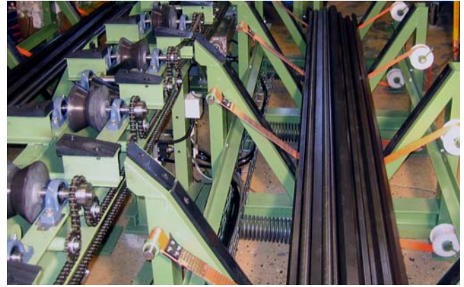
A combined feed system chain driven with easy drop incorporating technology from MAC and its subsidiary MA Nordic in Sweden.
