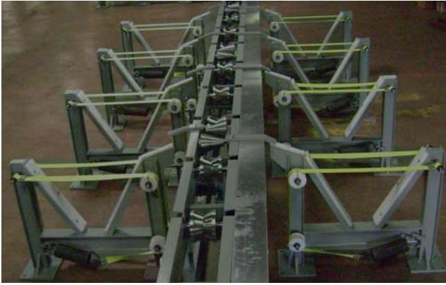
Outlet conveyor with accept/reject receiving pockets sorting to the left and the right.
