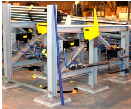
The picture above shows the stop arms on an incoming feed rack which can either hold back bundles or individual tube, bar, and billets based on the application.
