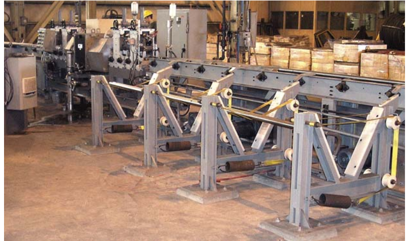
MAC' model 2063 Feed System accommodating material from 1" to 7 1/2" diameter, an Echomac® ultrasonic rotary on Dual Pinch Stands and FD-4 electronics with an AMFT Programmable Controller.
