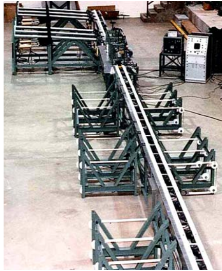
The picture shown above includes MAC's incoming feed rack (top left) with intermitant stop arms and a channel roll conveyor. The center section, which contains a test coil is installed between the incoming and outgoing channel conveyors. The receiving pockets, shown towards the bottom include the easy down hardware.
