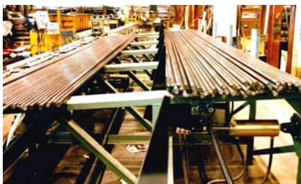
Intermediate Stop Arms hold back bars from a bundle that has just been broken out onto the Feed Rack in a bar mill.
