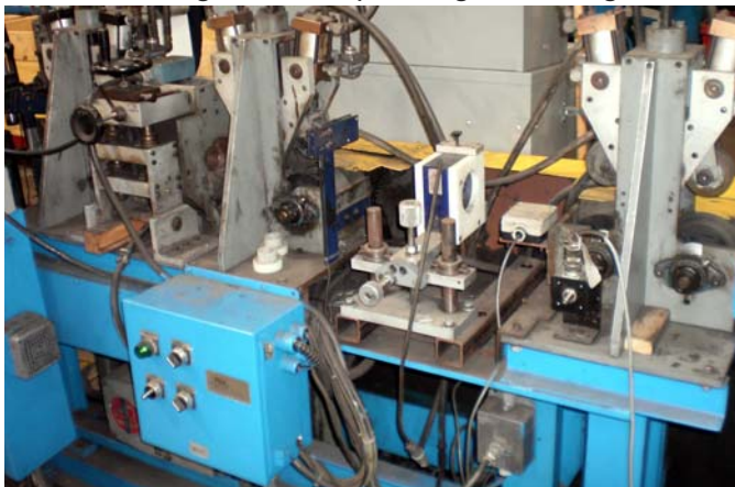
Coil Platform 352 on the left for defects and coil platform 30 towards the right for Sigma Phase.
