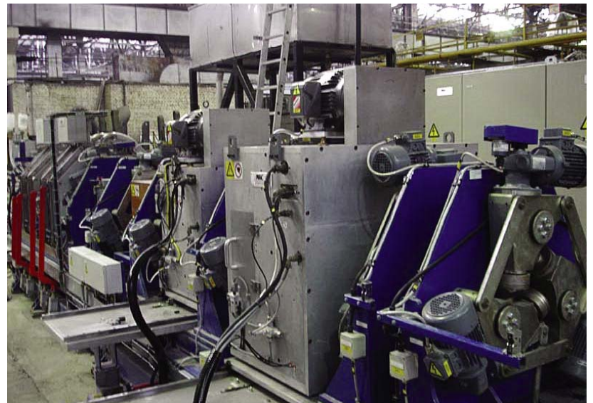
An installation at a large European tube mill, shown above, features both longitudinal and transverse Rotoflux® flux leakage rotary inspections. Inspections with this type of system are being conducted routinely at a 5% or 10% notch level on common OCTG products in a size range of 50 - 180mm (1.97" - 7") diameter. Inspection complies with API 5CT - Rev 8 specifications.
