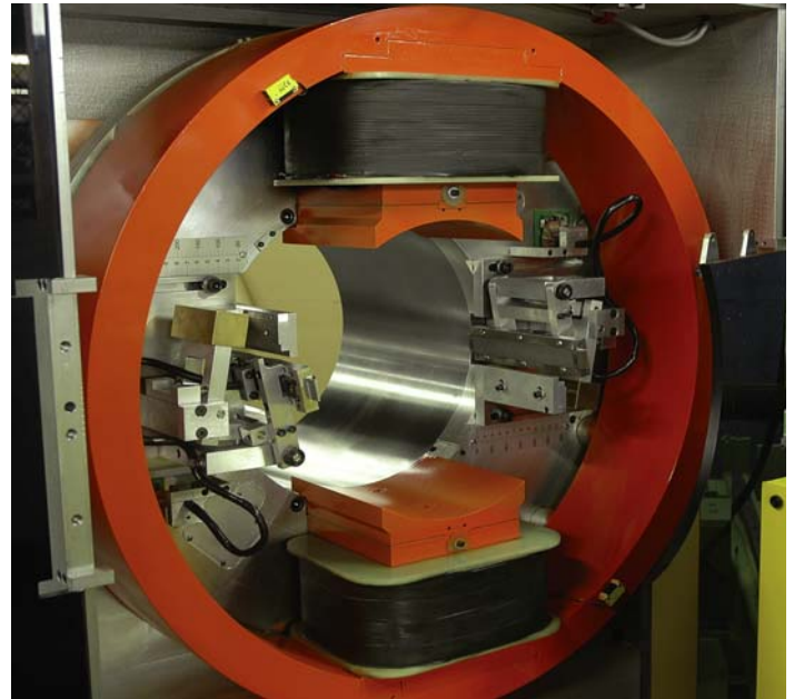
Rotoflux rotary headplate assembly with magnetizing coils on top and bottom. The probe assemblies which house the test probes are shown on either side. The rotary system is used to detect longitudinal defects such as seams, laps, and weld line defects.
