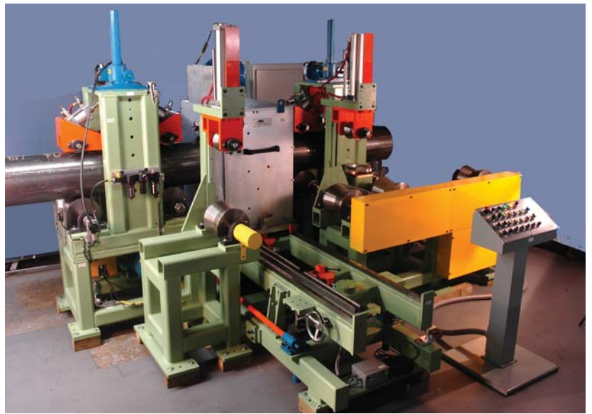
ROTOFLUX Type 1600 Rotary Head, Pinch Stands, Test & Calibration Stations, and Control Pedestal for a Longitudinal Flux Leakage Inspection system.
