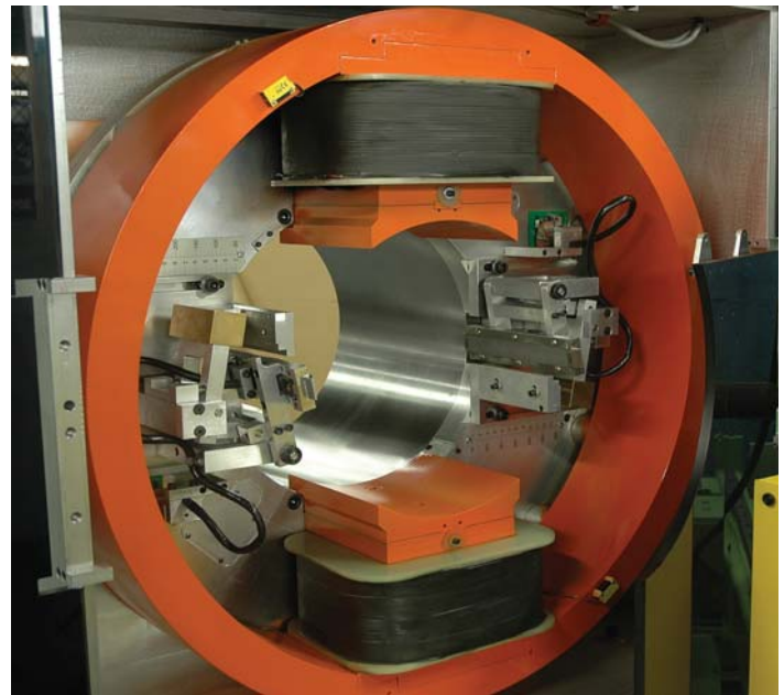
Rotoflux rotary headplate assembly with magnetizing coils on top and bottom. The probe assemblies which house the test probes are shown on either side. The rotary system is used to detect longitudinal defects such as seams, laps, and weld line defects.
