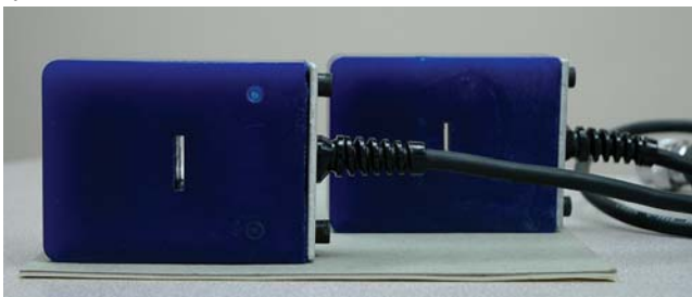
FIG 7 Coils for testing the above aluminum extruded tube
