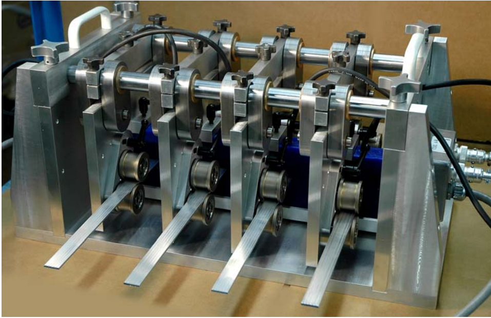
FIG 5- Is a Quad coil platform used on a multi line aluminum extruder. This system uses a single 4 channel Eric 6 High Frequency unit to simultaneously test for defects on the four lines. The difficult test here is for small defects that lie on the middle of the top or bottom surface, because of the low field density in this region and the presence of the varying finning that is extruded on the bore of this tube. Flaw down to .010" diameter are easily detected on the middle of the large flat surfaces.
