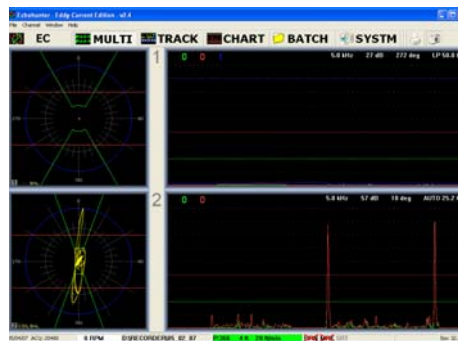
MultiMac Multi Screen, shows simultaneous polar and linear displays for two channels. Up to 2 channels, with all thresholds, can be displayed simultaneously.
