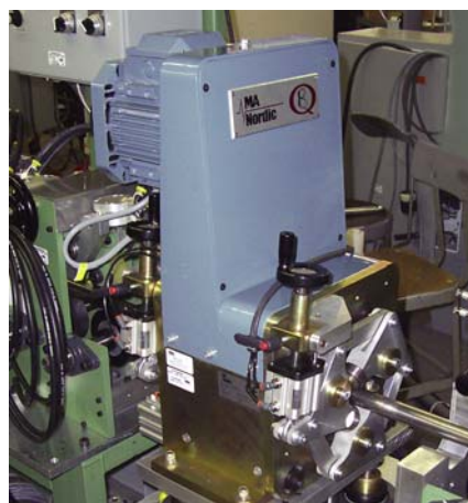
MAC's Rotomac ® E-Rotary test head, shown above, tests tube, bar or rod in continuous operations such as drawing, parts forming, or straight and cut. The inspection can operate automatically as defective pieces can be identified, then marked or rejected further down line, after the cutting and forming operation. Models for small diameter rod and wire are also available.
