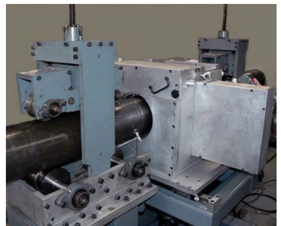
Shown above is the Model 750 Rotomac® rotary test head for inspecting 7-1/2" (190.5 mm) diameter cut lengths, often in-line with straighteners or installed in a separate test station. Installations can be completely automatic, including marking and sorting devices. The rotary is usually mounted in conjunction with MAC Slide/Elevating and Drive Mechanisms to position the rotary housing and move the material accurately through the test head.
