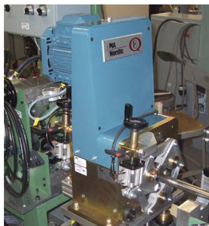
MAC's Rotomac® E-Rotary test head, shown above, tests tube, bar or rod in continuous operations such as drawing, parts forming, or straight and cut. The inspection can operate automatically as defective pieces can be identified, then marked or rejected further down line, after the cutting and forming operation. Models for small diameter rod and wire are also available.
