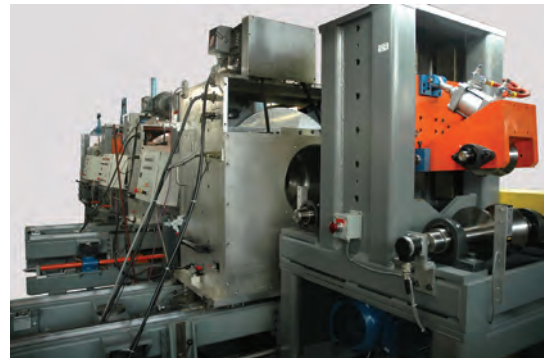
A combination Ultrasonic and Flux Leakage (MFL) system for inspecting large diameter, heavy wall oil country tubular goods (OCTG). The system includes a UT rotary, a transverse MFL and longitudinal MFL.
