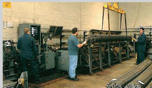
Steel bar being eddy current tested in MAC's Ohio Lab
