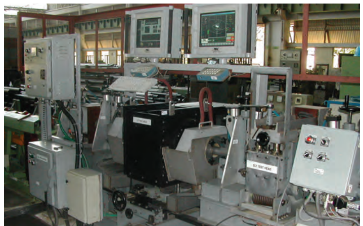
Combined encircling coil eddy current and ultrasonic test on welded steel tube. Eddy Current coil is at right with the tall handle, UT transducers are in the black enclosure near center. Monitors for the Echomac FD-4 and Eddy Current instrument are at center, above.
