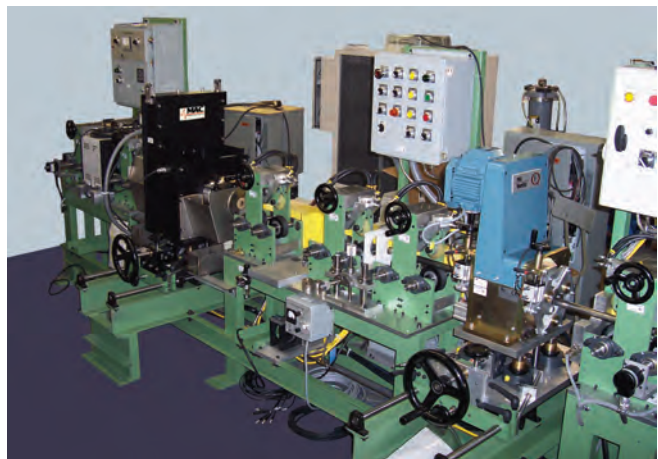
A combination Ultrasonic and Eddy Current inspection system for detecting defects in bar. The system is complete with a demagnetizer and a "V" Roll Dual Pinch test bench.
