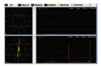
The Multi Screen above, shows simultaneous polar and linear displays for two channels. The screen for channel 2 demonstrates that a defect outside the acceptable parameters has been detected. Also shown here is the rotary speed, piece number, length, and ft/min (or parts per hour).
