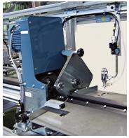
The parts are placed on a feed rack, where a release mechanism deposits one part at a time on the inlet conveyor. The part is fed through the eddy current rotary, where two probes rotate around the circumference of the part. This system is set up to inspect
